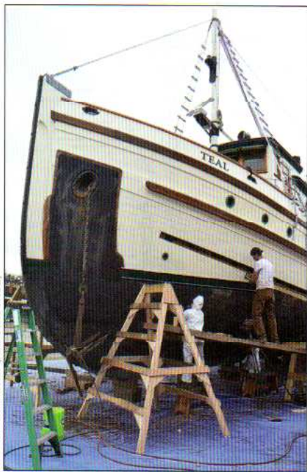
Above left —Since buying the boat in 2008, Kit Pingree has continued TEAL's maintenance and restoration. In 2016, the boat was hauled again at Port Townsend for additional work, mainly painting. Here, her 500-lb anchor is visible. Above right —In the latest haulout, a handful of planks needed replacement, exposing TEAL's heavy double-sawn frames.
