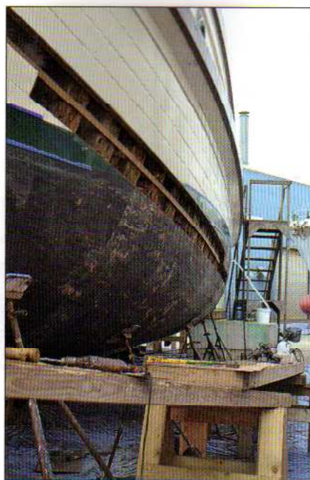
Above left —Since buying the boat in 2008, Kit Pingree has continued TEAL's maintenance and restoration. In 2016, the boat was hauled again at Port Townsend for additional work, mainly painting. Here, her 500-lb anchor is visible. Above right —In the latest haulout, a handful of planks needed replacement, exposing TEAL's heavy double-sawn frames.
