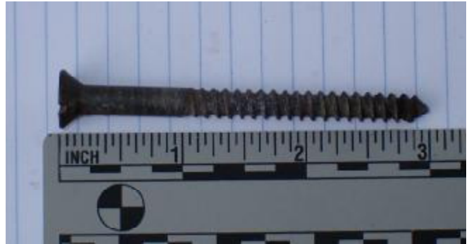
Galvanized, slot-head screw, 1/4"ø x 3".
