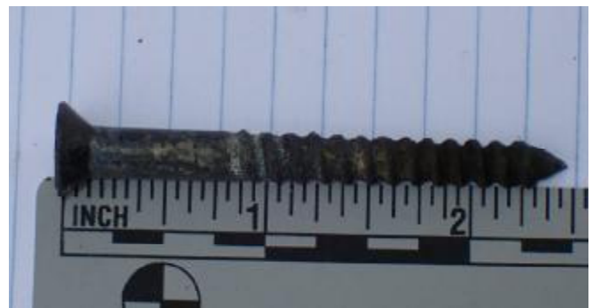
Galvanized, slot-head screw, 1/4" \phi x 2-1/2".
