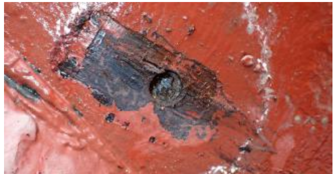
Galvanized, slot-head screw. Could not remove.
